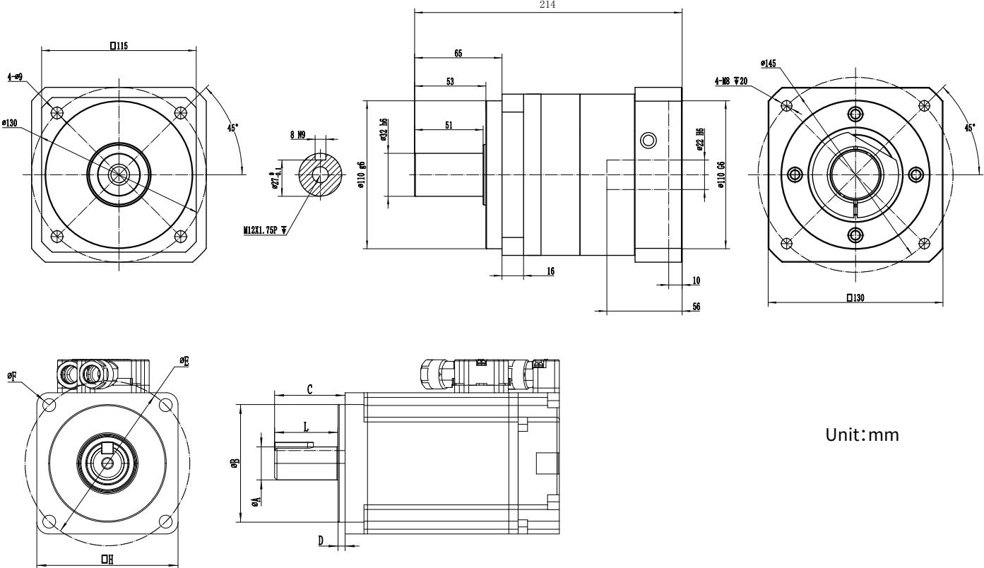
C: 马达轴长度。Length of motor output shaft.
